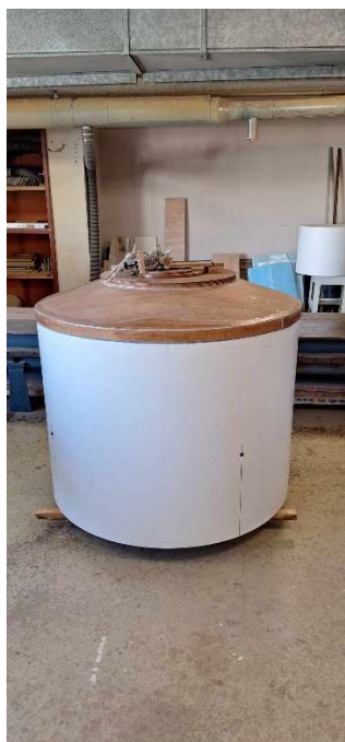
Figure 7: Construction process of the openings in the air oscillating chambers made from ply wood
