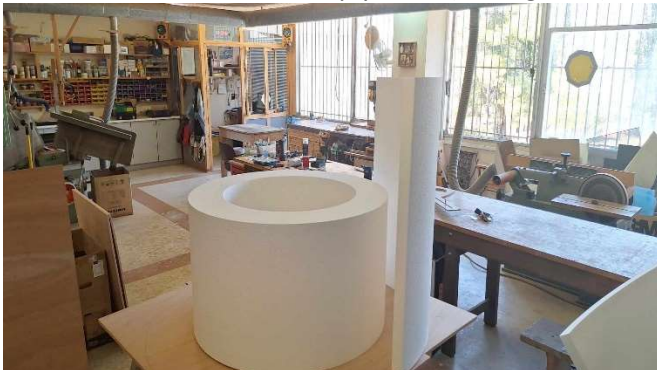
Figure 6: Construction process of the two coaxial cylindrical floaters made of expanded polystyrene
