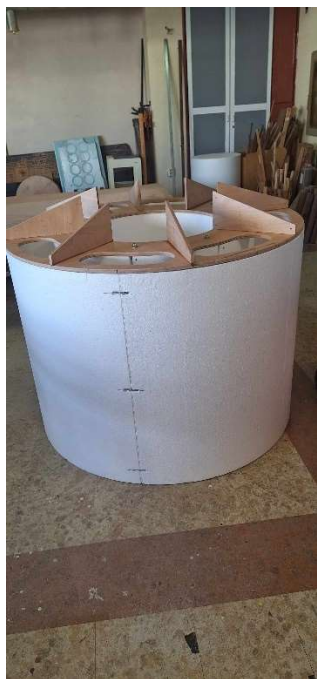
Figure 7: Construction process of the openings in the air oscillating chambers made from ply wood
