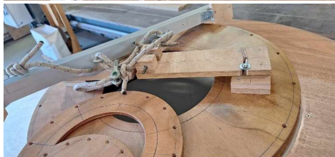
Figure 9: Construction process of the different orifices made from ply wood
