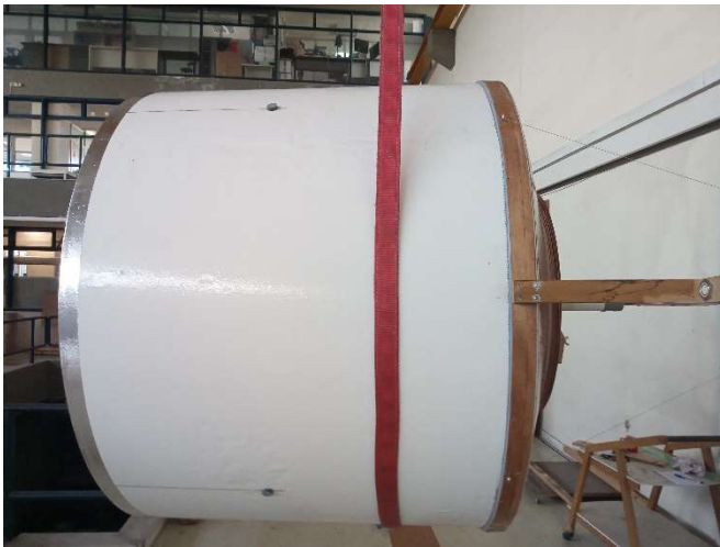
Figure 10. The initial vertical CG of the model measured experimentally
