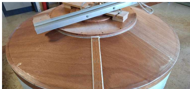
Figure 8: Construction process of the conical dome made from ply wood
