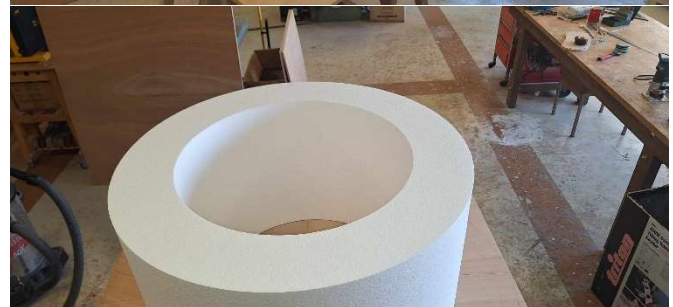
Figure 6: Construction process of the two coaxial cylindrical floaters made of expanded polystyrene
