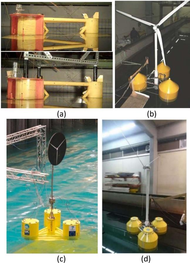
Figure 10. Hybrid OWC systems: (a) WindFLOAT model in the wave tank (adopted from Ref. [172]); (b) tension leg hybrid platform in the wave tank (adopted from Ref [174]); (c) MUP converter in the wave tank (adopted from Ref. [175]); (d) REFOS platform in the wave tank (adopted from Ref. [176])
