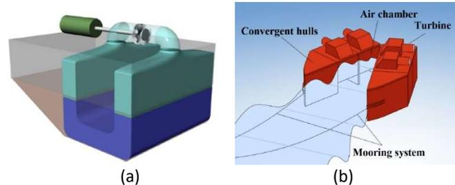
Figure 9. OWC of a random geometry: (a) 3D representation of the UGEN converter (adopted from Ref. [149]); (b) 3D representation of the MCOW converter (adopted from Ref. [151])
