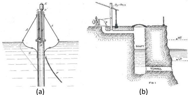
Figure 1: First known patent to extract energy from ocean waves: (a) whistling buoy patented by J.M. Courtney (adopted from Ref. [6]); (b) Bochaux-Praceique power system (adopted from Ref. [10])
