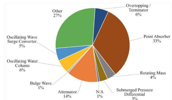
Figure 3: Distribution of wave energy technologies according to EMEC's WEC classification (adopted from Ref. [17])
