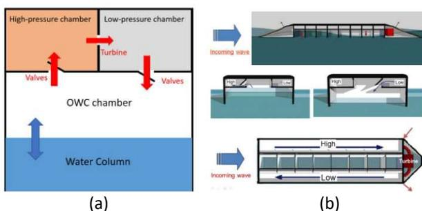
Figure 6. Spar-type and square- type oscillating water column models: (a) Tupperwave converter (adopted from Ref. [80]); (b) Seabreath WEC (adopted from Ref. [93])
