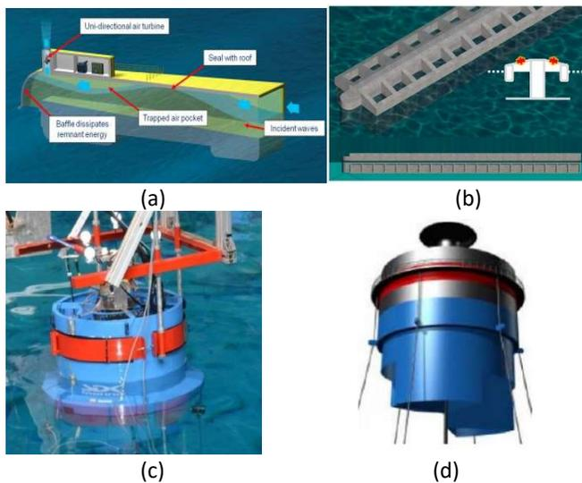
Figure 5. Oscillating Water Column prototypes that are in a design process: (a) OWEL wave energy converter (adopted from Ref. [45]); (b) KNSwing floating WEC (adopted from Ref. [47]); (c) SDK Wave turbine (adopted from Ref. [49]), (d) MRC1000 floating buoy (adopted from Ref. [52])
