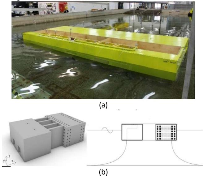
Figure 7. Breakwater with integrated OWC devices: (a) Scaled down breakwater in the test basin of Australian Maritime College (adopted from Ref. [119]); (b) Visual representation of a perforated floating breakwater (adopted from Ref. [128])
